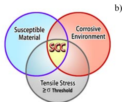
Figure 1. Schematic representation of stress corrosion cracking (SCC) phenomenon.
